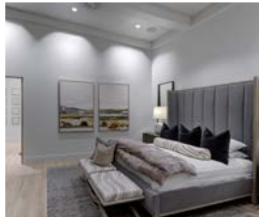
Scallops placed too low on wall with cause a "cave effect"
